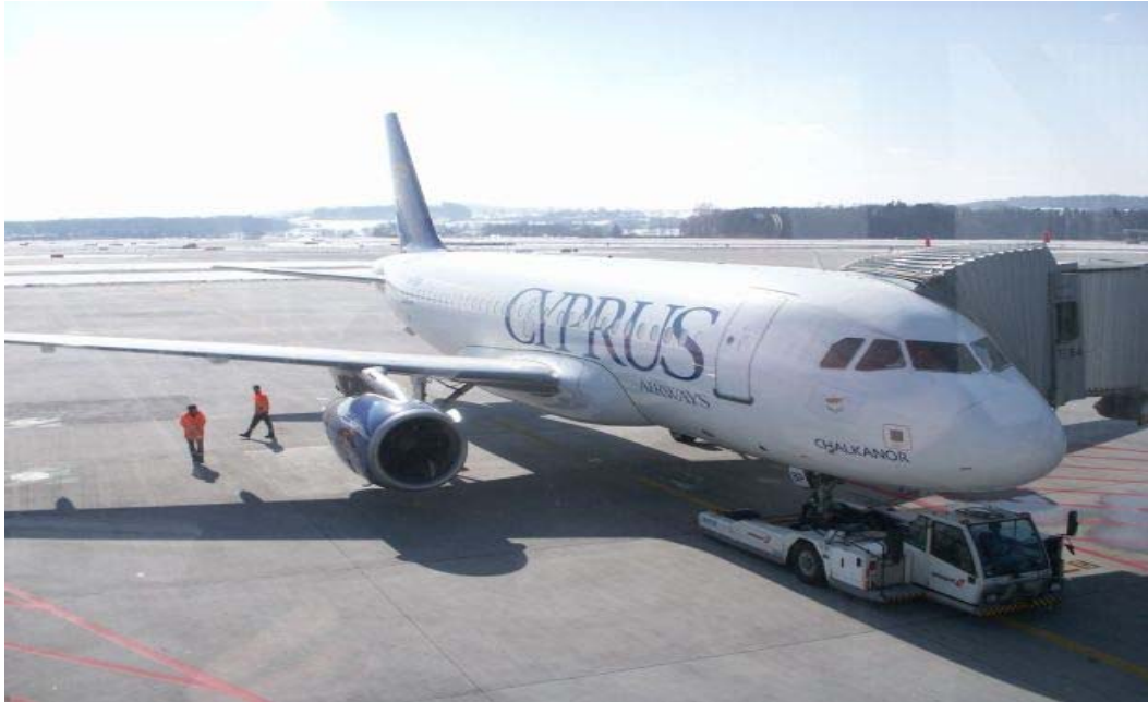
Picture 2.1 An A320 with TBL pushback truck at the gate, with the ground handling staff
