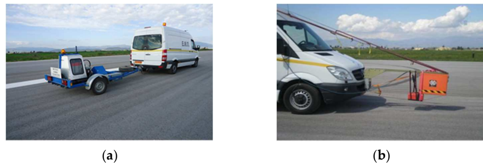
Figure 2. NDT measurements: (a) FWD; (b) GPR.
