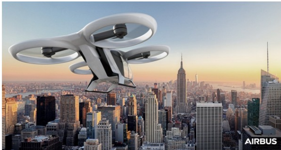
City Airbus, 4 passengers, endurance: 15 min. (Airbus 2017a)
